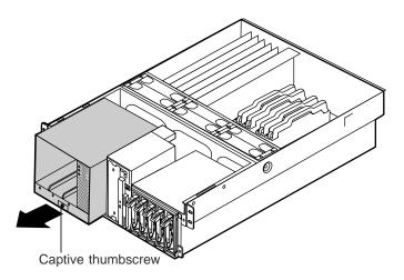
**8** Tilt the power supply forward and lift it up and back to clear the tab on the bottom of the chassis.
